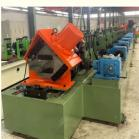
45 Degree Cutting purlin machine, High-speed Purlin Roll Forming Machine
